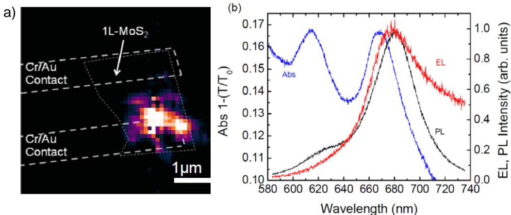
**Figure 1.** (a) False color image showing EL emission in the vicinity of a contact edge. The positions of Cr/Au contacts are highlighted by thick dashed lines (white) and the MoS<sub>2</sub> layer is indicated by thin dashed lines (grey). Absorption (Abs), EL, and PL spectra on the same 1L-MoS<sub>2</sub>.
